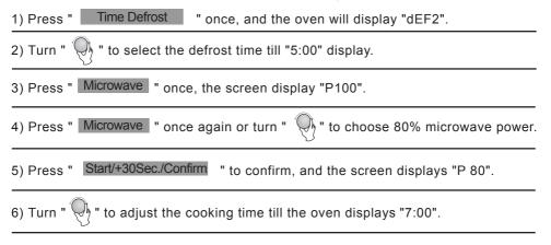
7) Press "Start/+30Sec./Confirm " to start cooking, and buzzer will sound once for the first section, defrosting time counts down; buzzer will sound once again entering the second cooking. when cooking finish, buzzer sounds five times.
