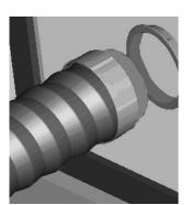
5. Insert the flexible pipe thus mounted into the rear of the air conditioner.
