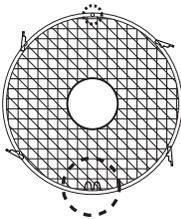
2. Press down all the Buckles to fasten the Front Guard with the Rear Guard. At the Screw Holes, tighten the separated screw and nut.
