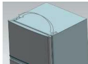
10) Set the top door right position,fix the top-hinge and the cover.
