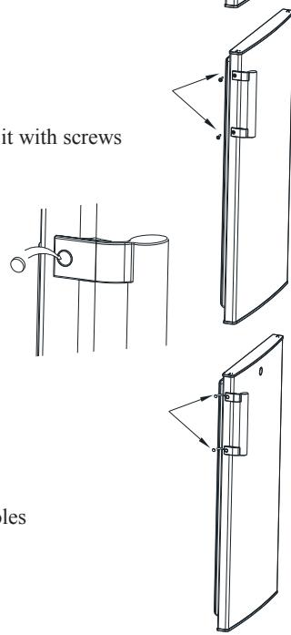
Step 3: Cover screw caps of the handle into screw holes
