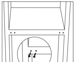
11. Lie down the rear of cabinet on a soft pad. And unscrew the bottom hinge and leveling foot.
