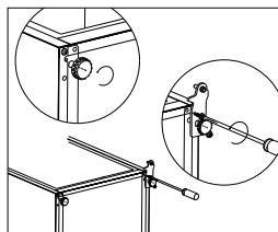
12. Stand up the unit and put the door on the bottom hinge. Make sure the bottom hinge core is inserted in the door hole. Then move the hinge hole cover of bottom door from left side to right side.
